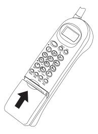
The built-in Memory Backup feature allows up to 3 minutes to disconnect the old battery pack and install a new one without losing any numbers stored in memory.
